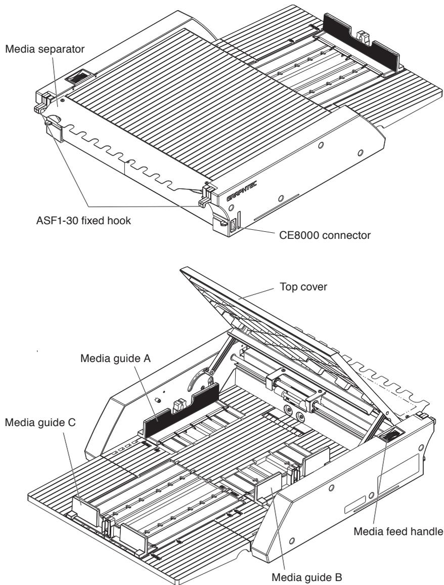
ASF1-30 fixed hook .....This is a hook to secure the ASF1-30 and CE8000-40.
