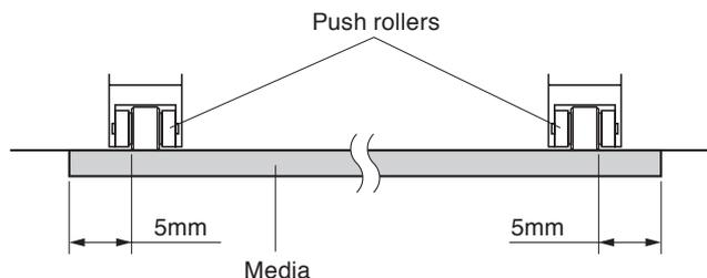
3. After adjusting the position of the push roller, turn the media feed handle to eject the media.
