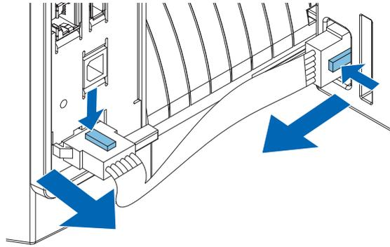
4. Raise the ASF1-30 fixing hook, and then remove the ASF1-30 toward the rear.
