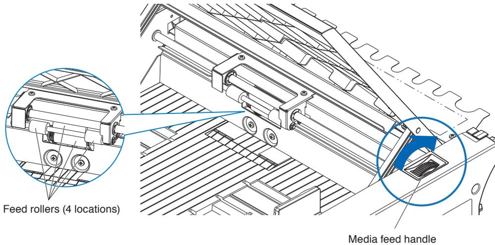
2. Clean the feed rollers by lightly pressing a soft cloth soaked in alcohol (95% or more) against the feed rollers.
