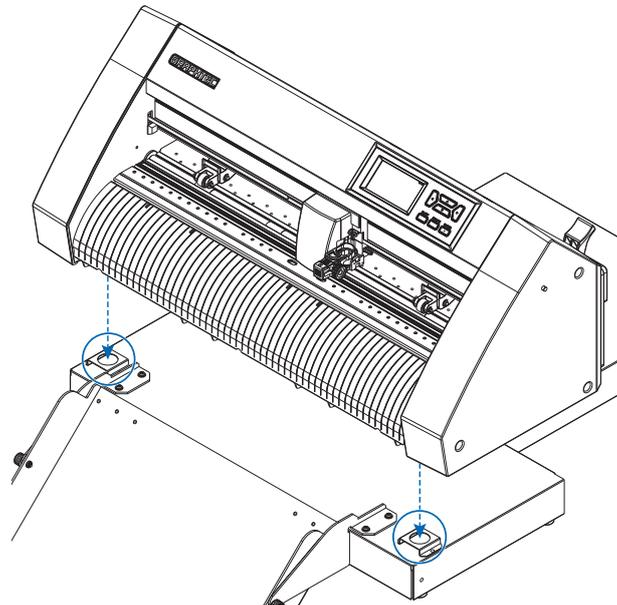
2. After installing the CE8000-40, press the CE8000-40 in the direction of the arrow in the figure below.
