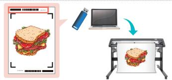
Automatic identification of cutting data with the dedicated barcode avoids cutting wrong data.
